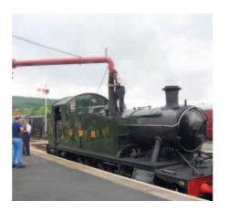
A steam train derives its power from an engine which produces steam in a boiler, usually fuelled by coal. As the fuel heats the water in the boiler, steam is generated and that is used to drive the locomotive, as well as working the whistle, brakes, pumps and heating throughout the carriages.
